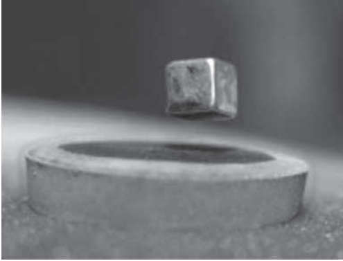
Fig. 3: A magnet levitating above a high-temperature superconductor, cooled with liquid nitrogen.
